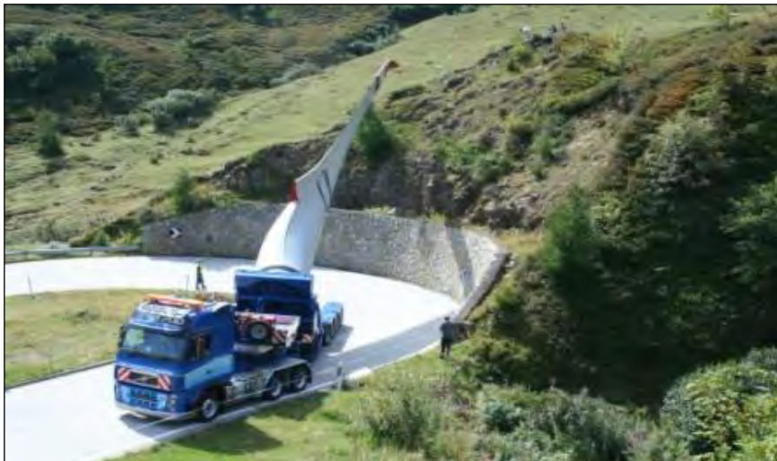
Plate 4-4 Blade adaptor transport system
